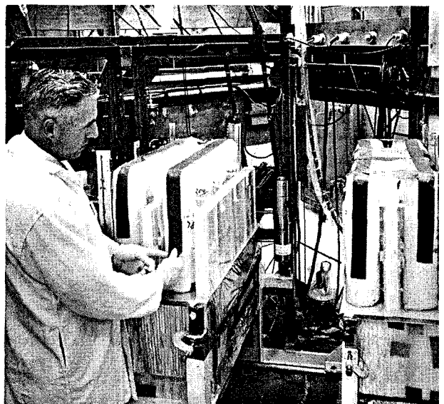
Fig. 1. 16-Bottle moderated unreflected array of 233 U solution.
