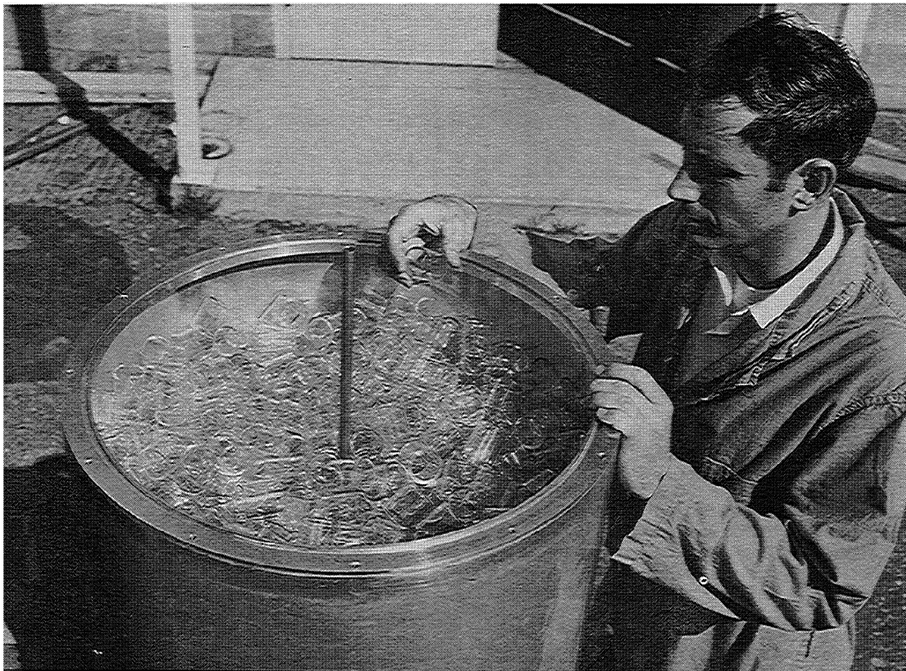
Fig. 2. Experimental vessel loaded with glass raschig rings.
