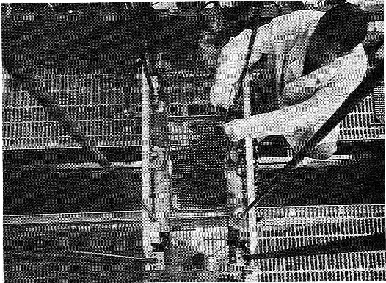
Fig. 1. Partially loaded lattice of FTR fuel pins immersed in water.
